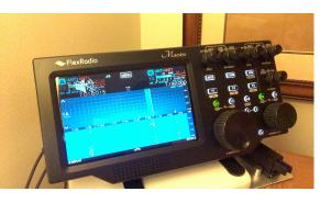
Jason, KY9I, shared with the Club how to use the Flex Maestro to remote control his rig at home from the WKCTC meeting room. The Flex 6600 is connected to an end fed half wave antenna in his shack and to his home network with an ethernet cable. The Maestro was connected to the College network with an ethernet cable, although the unit
